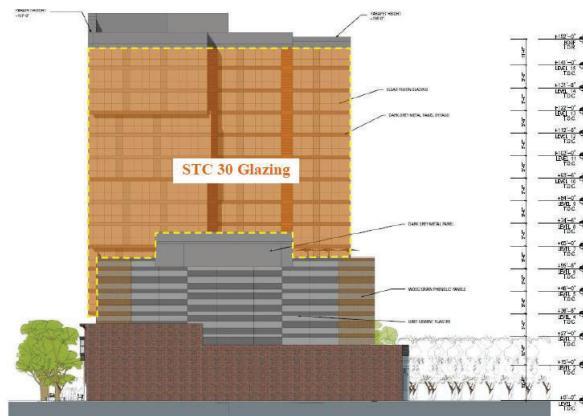
Figure 25 North Side of Building Window STC Ratings
